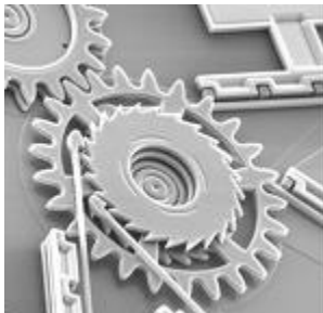
MEMS escapement and gears etched in silicon
