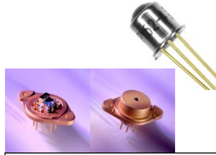
Laser welded TO-18 package, above, and integrated circuit in TO-3 package shown open and welded closed.
