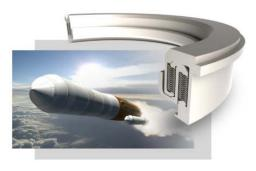
For NASA's Space Launch System, Flexial designs and builds the J-2X turbopump lift-off seal. This is a high-performance sealing technology to prevent leakage of hydrogen while the engine turbopump spins at up to 30,000 revolutions per minute; perhaps one of the most demanding face seal applications ever.
